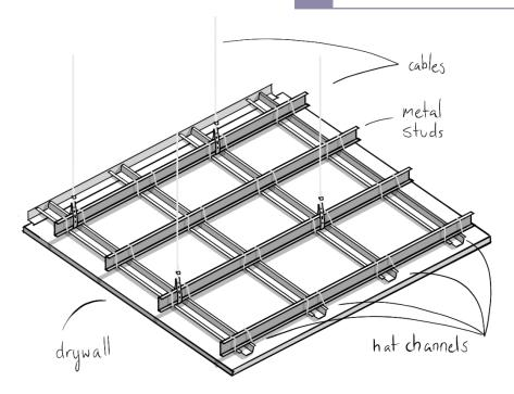
You don't want your drop ceiling to fully touch your walls. Leave the drywall hanging about 1/4" away from the walls and fill in the gap with sound caulk. You can then put silicone caulking over that to serve as a moisture barrier.
