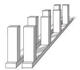
Double-stud walls have separate base plates, separate top plates, and separate studs. You only construct the outer walls on one side of each set of studs, but two walls are separate and never touch. Because you've created an actual air gap, this has a higher STC rating than either single or staggered stud walls.
