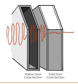
It's easy to get confused here and think that hollow-core is what you want, since you have an air gap on the inside. However, since the door material is all connected, it's not a 'true' air gap, and is much more akin to a single stud wall. Also, since mass is so important in blocking sound, standard hollow-core doors will let A LOT of noise through.
