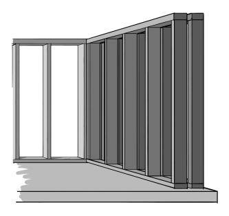
You should tear out your ceiling (remember the lesson of gutting your space) and put your top plates directly into your joists. You're going to want to extend your drywall all the way to your roof so you don't have a weak point going through your ceilings. As a result, you'll need to tear out large portions of the ceiling no matter what. We recommend tearing out the whole thing.
