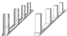
Metal studs are more expensive in both materials and installation, but if you aren't doing double-stud walls they're better for soundproofing (with a higher STC rating).
