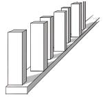
Staggered stud walls share a wider base plate and top plate, but the studs are offset, meaning the walls on either side don't touch. This is more soundproof, with a higher STC rating, than single studs, but the baseplates and top plates still connect the studs, so there is still a decent amount of vibration conveyed through the system.
