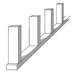
Single stud walls have one baseplate, one top plate, and a single set of studs running vertically between them. Because they have no air gap in them, these yield the least soundproof walls. You can combine single stud walls with sound channeling for a more soundproof setup, which we'll discuss later.
